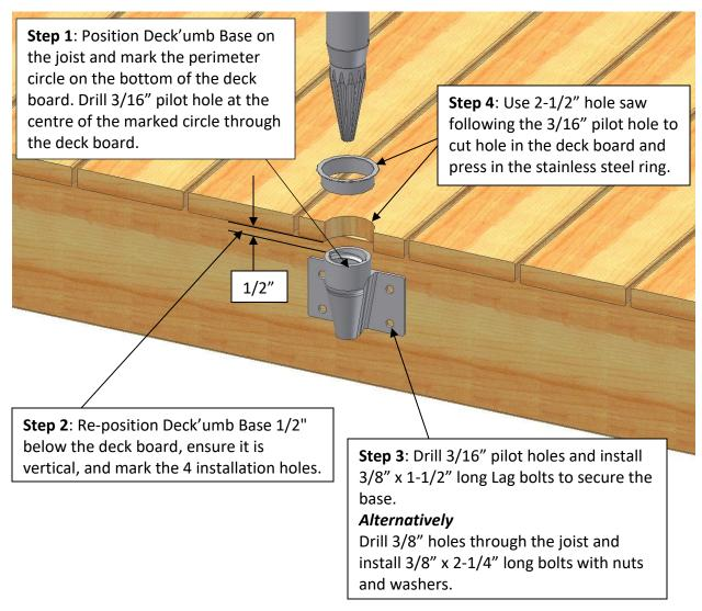
**Step 5**: Insert Deck'umb holder and line up the pin with the slot openings. Rotate the holder clockwise until it stops and then rotate counter-clockwise to lock it in the base.
